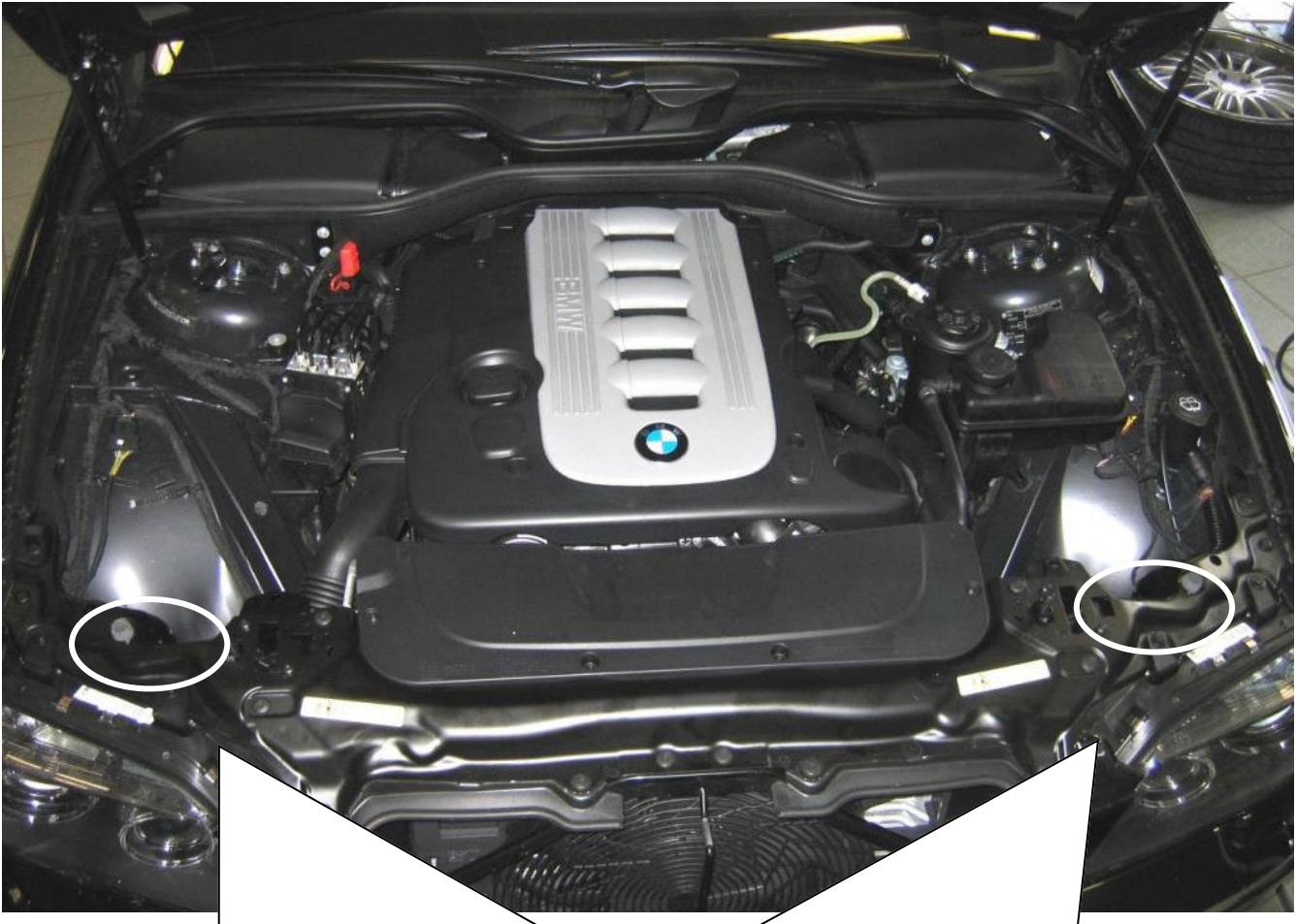
Montageort VA Elektroniksatz / Assembly site front axle electronic kit
