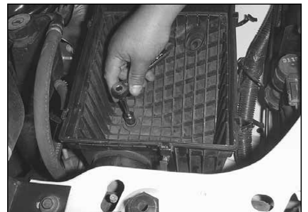
5. Using a 1/2" socket, loosen and remove the three bolts that secure the air box base.
