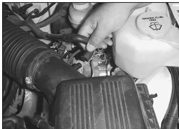
3. Disconnect the factory crank case vent at the air box.
