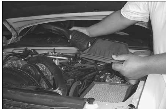
4. Unclip the six over center clamps and remove the complete upper intake assembly as shown.
