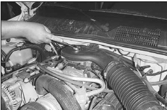
2. Loosen the nut at the intake plenum as shown.
