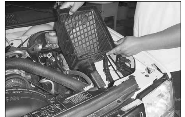
6. Remove the air box base as shown. NOTE: K&N Engineering, Inc., recommends that customers do not discard factory air intake.
