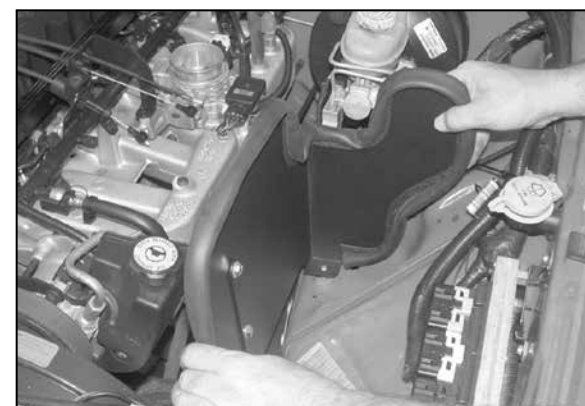
8. Install the heat shield into the vehicle as shown.
