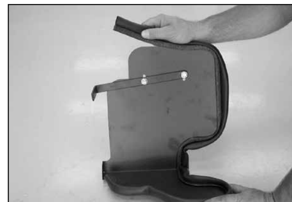
7. Install the trim seal to the heat shield as shown. Trim as needed.
