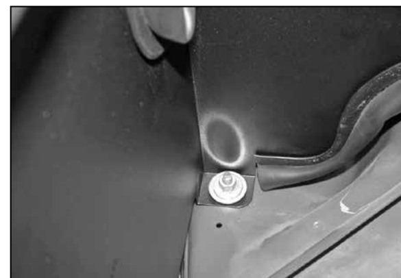
9. Secure the heat shield to the original air box mounting stud using the provided washers, and the nut removed in step 5. Do not tighten completely.
