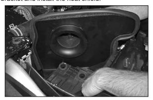
28a. On 2004 and later vehicles, lift up the air boxevap bracket and install the heat shield as shown.
