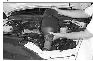
9. Pull upward firmly and remove the air cleaner. NOTE: K&N Engineering, Inc., recommends that customers do not discard factory air intake.
