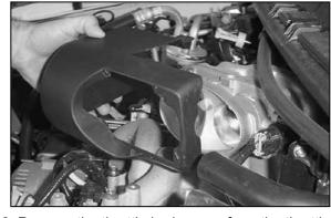
8. Remove the throttle body cover from the throttle body as it will not be reused.
