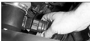
38. Reconnect the primary mass air sensor electrical connection.
