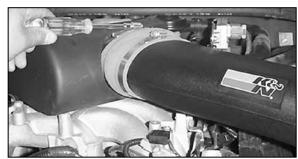
31. Tighten the hose clamp on the hump hose at the throttle body.
