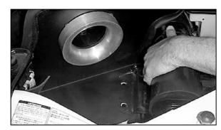
28. Lift up on the evaporative canister mounting bracket and install the heat shield.
