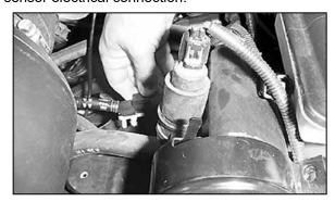
3. Detach the mass air sensor wiring harness from the inner fender apron.
