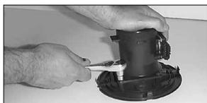
19. Loosen and remove the bolts that secure the mass air sensor to it's retaining plate.
