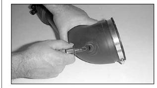
22. On models equipped with an external air temperature sensor, remove the air temperature sensor from the stock intake tube.
