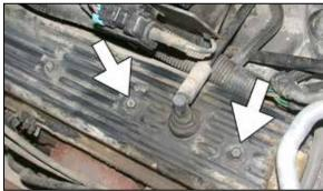
15. Remove the two valve cover bolts as shown.
