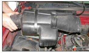
4. Loosen and remove the two bolts that secure the air inlet/resonator, then remove the assembly as
