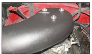
20. Reinstall the K&N® intake tube and secure it with the provided washers and nylock nuts.
