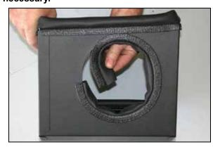
13. Install the short piece of trim seal to the heat shield as shown.
