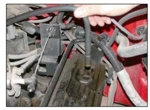
5. Remove the crank case vent line from the valve cover as shown.
