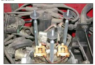
11. Install the three flat washers onto the throttle body studs as shown.
