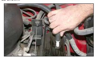
24. Install the silicone hose onto the vent on the K&N® intake tube, then push the hose mender into the grommet on the valve cover.
