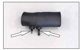
6. Install the two provided vent fittings into the K&N<sup>®</sup> intake tube as shown.
