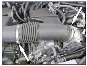
4. Loosen the two hose clamps securing the factory intake tube to the throttle body and air filter housing and then remove the factory intake tube.
