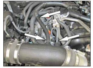
11. Install the crank case vent hose assembly into the factory crank case vent hose and then connect the open end to the fitting installed into the  $K\&N^{\mbox{\ensuremath{\mathbb{R}}}}$  intake tube. Connect the factory fuel pressure regulator vent hose into the fitting installed into the  $K\&N^{\mbox{\ensuremath{\mathbb{R}}}}$  intake tube.
