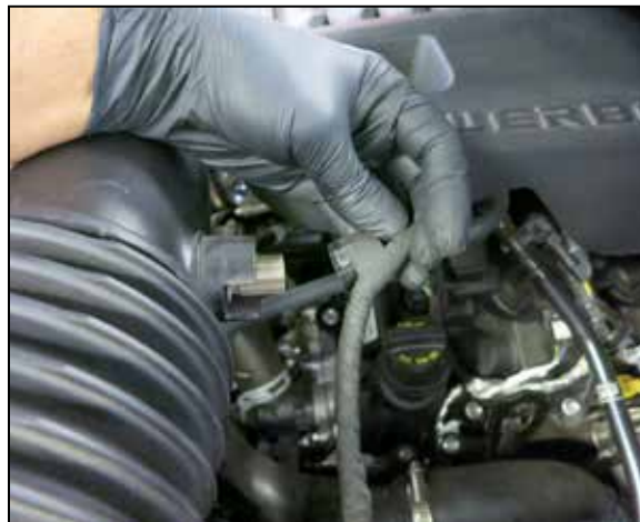
3. Disconnect the IAT sensor electrical connection.
