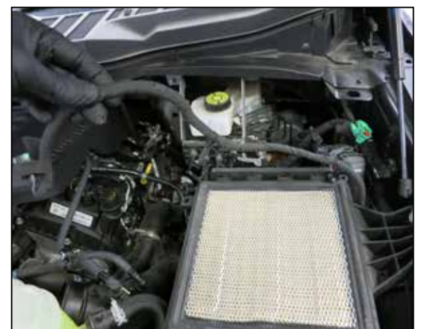
6. Unhook the IAT sensor wiring harness from the lower air filter housing.
