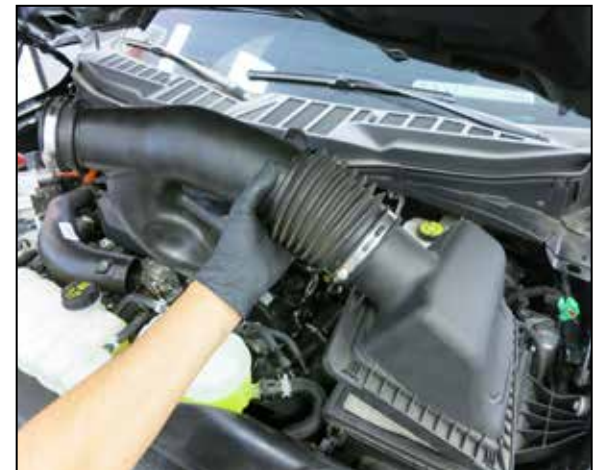
5. Lift the upper air filter housing and intake tube up and out of the engine compartment.
