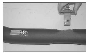
20. Install the mass air sensor assembly into the K&N® intake tube with the supplied hardware as shown.
