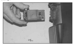
17. Remove the two mass air sensor retaining screws and then remove the mass air sensor from the factory air box.
