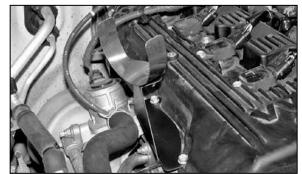
15. Install the tube mounting bracket assembly onto the valve cover using the factory bolts removed in step #14.
