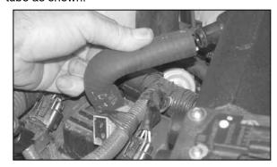
25. Install the provided crank case vent hose onto the valve cover port and then onto the K&N<sup>®</sup> intake tube as shown.
