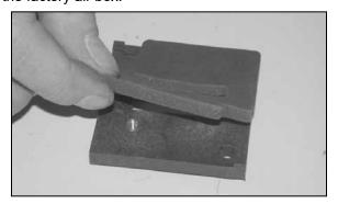
18. Install the supplied gasket onto the mass air sensor adapter as shown.
