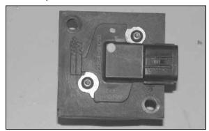
19. Install the mass air sensor into the K&N® mass air adapter and secure with the provided bolts as shown.
