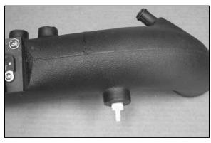
21. Install the supplied npt fitting into the K&N<sup>®</sup> intake tube as shown.
