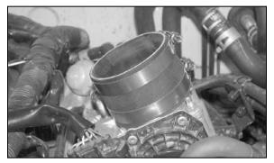
16. Install the provided silicone hose (08756) onto the throttle body and secure with the provided hose clamp.
