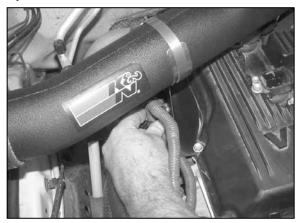
30. Clip the mass air sensor wire harness retainer into the tube-mounting bracket as shown.
