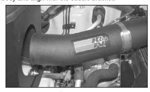
23. Secure the K&N® intake tube to the saddle bracket with the provided hose clamps. Also tighten the hose clamp securing the intake tube to the throttle body.
