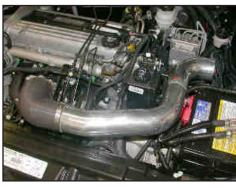
24. Install the K&N® intake tube into the silicone hose at the throttle body and align with the tube mounting bracket installed in step #21a. Secure the intake tube with the provided hose clamp and hardware.
