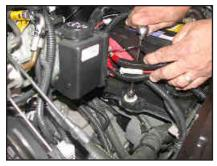
17. Reinstall the battery hold down block as shown.
