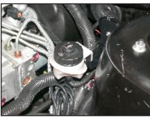
19. On manual transmission vehicles slide the fluid reservoir onto the bracket from step 18 as shown.
