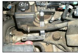
21a. Install the tube mounting bracket (070105) onto the stud and secure with the nut from the previous step.
