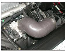
20. Install the silicone hose and hose clamps onto the throttle body as shown.
