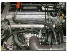
26. Connect the one end of the provided silicone hose to the vent on the cam cover, then, connect the other end to the vent on the K&N® intake tube and secure with the provided hose clamps as shown.
