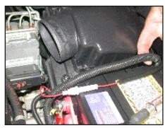
10. Unclip the wire harness from the air cleaner cover as shown.
