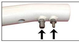
22. Install the two provided 1/4" NPT fittings into the K&N® intake tube as shown.
