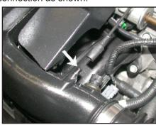
3.Disconnect the vent hose from the stock intake tube as shown.
