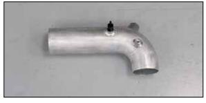
13. Install the provided vacuum fitting into the  $K\&N^{\circ}$  intake tube as shown.
