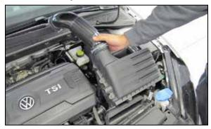
4. Lift up the air filter housing to dislodge it from the mounting grommets and then rotate the assembly up from the rear to disengage it from the fresh air intake and remove it from the vehicle. NOTE: K&N Engineering, Inc., recommends that customers do not discard factory air intake.
