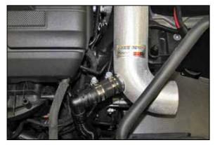
19. Connect the secondary air hose onto the Quick disconnect fitting and connect the vacuum line to the fitting installed into the K&N<sup>®</sup> intake tube. NOTE: On vehicles not equipped with a secondary air tube, install the provided cap into the fitting installed on the K&N<sup>®</sup> intake tube. On some models it may be necessary to replace the factory vacuum line with the longer vacuum line provided.
