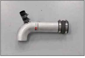
16. Install the remaining coupling hose (08185) onto the K&N<sup> $\otimes$ </sup> intake tube as shown.
