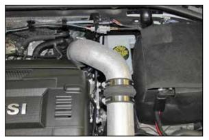
18. Install the rear K&N<sup>®</sup> intake tube into the coupling hose on the front intake tube and then into the coupling hose at the turbo inlet, adjust the tubes for best fit and then secure with the provided hose clamps.
