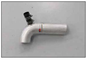
15. Install the secondary air fitting onto the  $K\&N^{\circledast}$  intake tube as shown.
